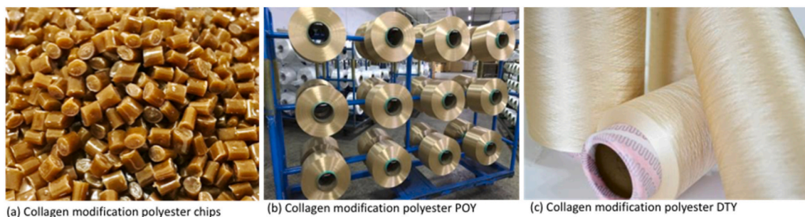
Fig. 4. Champagne appearance of collagen modification polyester products at different stages: (a) slices, (b) POY and (c) DTY.
